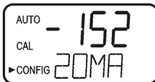
This setting will be slightly different on each instrument as each CLX-XT will be factory set to 20.00mA.
