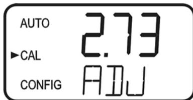
5. The screen will show the current reading on the CLX-XT. Using the  $\blacktriangle$  and  $\blacktriangledown$  buttons adjust the reading to agree with the laboratory method or portable photometer.
