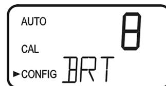
Change the brightness by pressing the ▲ or ▼ button. When the desired brightness has been selected, press the ↵ button.
