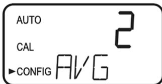
helps smooth out large changes and eliminate reading spikes. After 3 consecutive readings, it is assumed that the large change in the readings is "real", and the filter will be disabled. For example, the change between reading 1 and 2, and readings 2 and 3 will be limited to 20%, but the change between readings 3 and 4 will not be limited.
