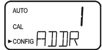
Press the  $\leftarrow$  button to continue on and select the desired instrument address using the  $\blacktriangle$  or  $\blacktriangledown$  buttons. Once the selection is satisfactory, press the  $\leftarrow$  button.
