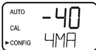
This setting will be slightly different on each instrument as each CLX-XT will be factory set to 4.00mA. Press the **↵** button when adjustments are complete to save this setting and move on to the 20mA adjustment.
