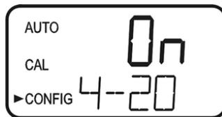
If the 4-20 mA output was turned **On**, prompts to set the 4mA (4MA) and 20mA (20MA) chlorine limits will be displayed. There will also be a menu to adjust the error level (ERLV). The first prompt will be the chlorine limit assigned to the 4 mA output level:
