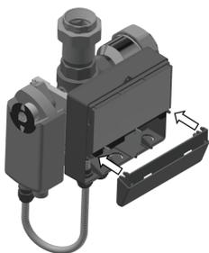
18. Put the wiring cover back on and tighten the 2 screws.
