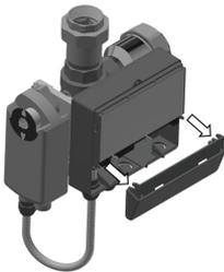
5. Pull the wiring cover straight out from the wiring chamber.
