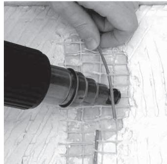
**Step 3.4.** With either type of jacket, if it doesn't easily pull off you may need to use your heat gun to gently warm the slug, which should soften and loosen it for you. Use the heat gun (set to about 500°F) and move the gun back and forth under the jacket slug for about 3 or 4 seconds, or until it can be easily removed.
