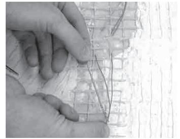
**Step 3.9.** Pull the braid straight out to make it into a pigtail.
