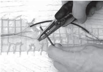
**Step 4.13.** Use the 16 AWG setting on the wire strippers to strip off exactly 1/2" of the insulation from both ends of the jumper wires.
