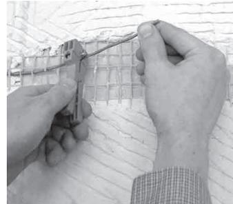
Some of our products have an "XLPE" jacket that is a somewhat hard material that can be lightly "scored" with a scoring tool or sharp blade. Use the scoring tool to carefully score the jacket about 2.5" from the end of each lead. Do this by placing the cable lead into the V-notch of the tool and rotating the tool only one or two revolutions around the cable. Do not place any additional pressure on the tool head to cut deeper. Let the tool apply its own spring-loaded pressure.
