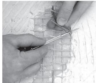
**Step 3.8.** Use the small screwdriver, paper clip, fingernail, or similar blunt instrument to pry between the braid and make an opening through which to pull the heating wires. Pull each wire through the braid.
