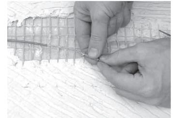
**Step 4.6.** Loosen the braid by pushing back on the braid about 1/2", causing the ends of the heating wires to be exposed. **Note:** Some of our heating cables do not have a braided ground shield. These cables will have a ground drain wire and a foil wrap. Simply remove the foil and proceed to Step 4.10.
