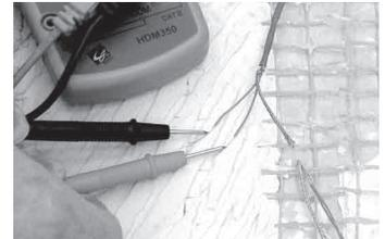
**Step 3.11.** Use the digital multi-meter and TDR at this repair location before proceeding. Check for any additional damage locations in the heating cable by "looking" in both directions. For assistance in using these instruments, consult the instructions that came with them.
