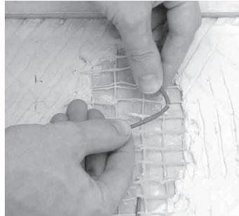
**Step 3.3.** Gently bend the cable at the score to break through the jacket all the way around the cable, then pull off the slug
