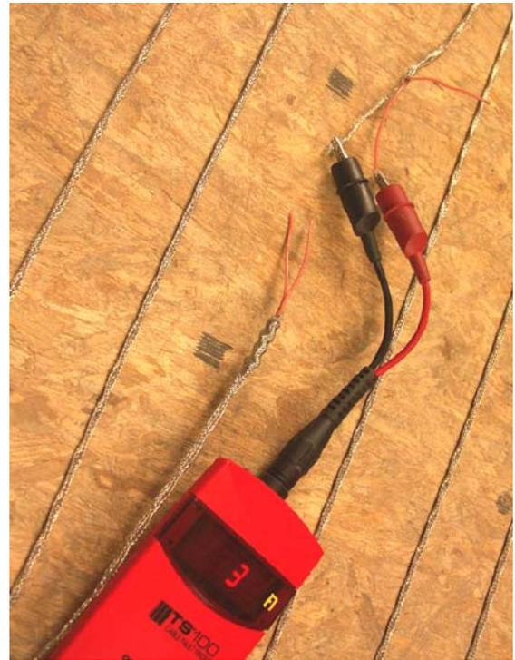
This shows the Fault Finder connected at the floor where a wire has been prepped for splicing. This is recommended BEFORE the splice is installed, in this case the meter shows another problem about 3 feet away. This is also a procedure that can be used to narrow in on a point of damage. Use of a digital ohm meter from this location is also advised. Test the cable in both directions.
