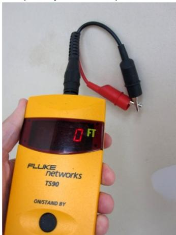
If the Fault Finder does not show steady values, or does not tone when touching test leads together, replace the "AA" batteries.
