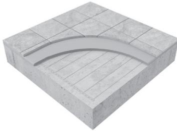
WarmWire over concrete slab floor
