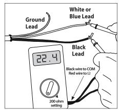
Press the test lead tips to the Black and White (or Blue for 240 VAC) power lead wires. This reading should correspond to the factory resistance range on the nameplate label attached to the Power lead.
