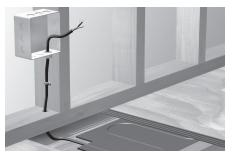
Drywall ceilings below the mats will require access doors or cover plates if there are joist bay junction boxes. An alternative is to install junction boxes with a cover plate in the space above.
