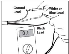
Readings between the Black and Ground and the White (or Blue for 240 VAC) and Ground power lead wires should measure "open", or "O.L", or the same as displayed when the test leads are not touching anything.
