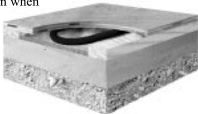
Install a high-temperature foil-faced foamboard insulation, such as Thermax<sup>®</sup> or equivalent, between the nailers. It is very important to carefully select the correct nailer and foamboard thickness, so that the Onix maintains continuous contact with the underside of the upper floor or subfloor, but isn't crushed or deformed.
