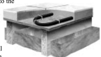
You must use a foil-faced insulation for this application, with the foil facing up. Allow a 2" minimum air space between the foil surface and the subfloor.
