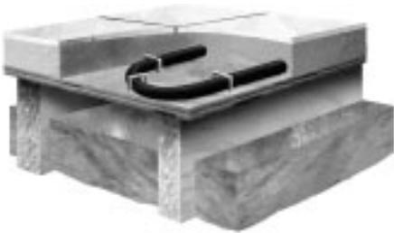
**Thin-slab and Slab Cap Applications**
