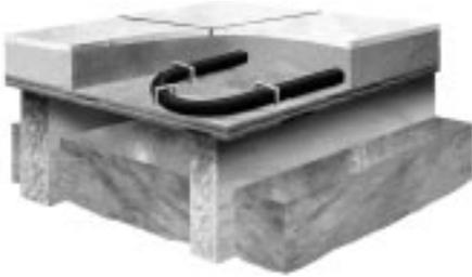
Some construction details call for a Thin Slab, or a lightweight concrete, to be applied above the subfloor. These applications offer increased sound quality to a room and an increased thermal mass to the radiant heating system. In some cases, thin slabs are used to act as a fire-stop from floor to floor.
