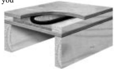
Install a high-temperature foil-faced foamboard insulation, such as Thermax<sup>®</sup> or equivalent, between the nailers. It is very important to carefully select the correct nailer and foamboard thickness, so that the Onix maintains continuous contact with the underside of the upper floor or subfloor, but isn't crushed or deformed.
