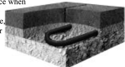
Onix is installed in a sand or crushed stone base, then secured with wire hooks every two feet along its length. A layer of sand is then placed over the Onix and compacted to provide a minimum of 1" coverage above the top of the Onix (more may be required depending on structural loading). The brick pavers are then installed on the compacted base material.
