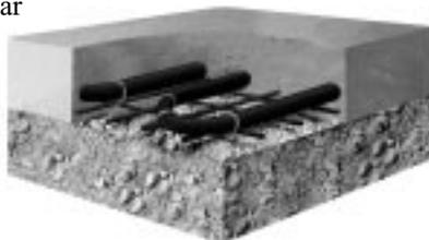
Install Onix midway in the slab or at a depth that will provide a minimum of 3" of concrete over the top of the Onix. More may be required depending on structural loading.
