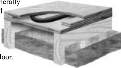
Always use a foil-faced fiberglass (foil facing up), leaving a 2" air gap between the foil and the underside of the subfloor. It is very important to select the correct nailer thickness, so that the Onix maintains continuous contact with the underside of the upper floor or subfloor, but isn't crushed or deformed.
