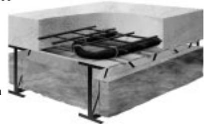
Use a foil-faced insulation for this application, with the foil facing up, and a 2" minimum air space between the foil surface and the steel deck.
