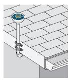
Roof Mounted Conduit fastened to fascia board
