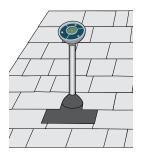
Roof Mounted Ensure water-proof installation with flashing boot or similar method
