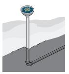
Ground Mounted Conduit run underground with a pole above surface
