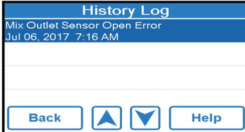
The screenshot shows a screen titled "History Log" with a blue header. Below the header, the text "Mix Outlet Sensor Open Error" and "Jul 06, 2017 7:16 AM" is displayed. The main area is empty. At the bottom, there are four buttons: "Back", an up arrow, a down arrow, and "Help".
