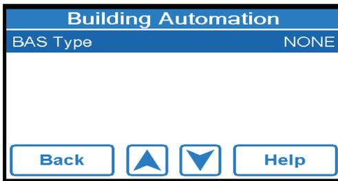
To change this setting press the “BAS Type” and adjustment screen will appear (as shown below).
