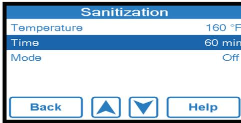
6. Using the slide bar or up and down arrows select the desired run time. Touch the **ACCEPT** icon to confirm the adjustment.
