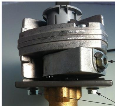
Armature Clamping Nut
