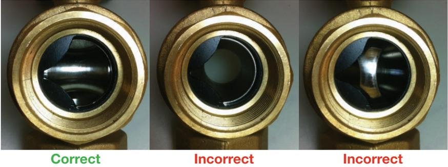
4. Once both the actuator and valve have been aligned “correctly” the actuator can be reinstalled onto the valve by sliding actuator over the valve stem until the actuator sits tight against the actuator support plate with the actuator positioned vertically as shown below.
